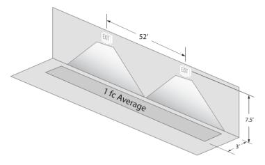
SAMPLE PHOTOMETRICS - 6' PATH OF EGRESS Using multiple NXFC units mounted at a typical 7.5' height delivers 48' on-center spacing with a 6' wide path of egress using 80/50/20 reflectances.
