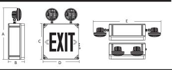
Single Face 17<sup>1/2n</sup> (445mm) 7" (133mm) 11<sup>3/4n</sup> (298mm) 11<sup>3/4n</sup> (298mm) 23<sup>1/4n</sup> (591mm)
